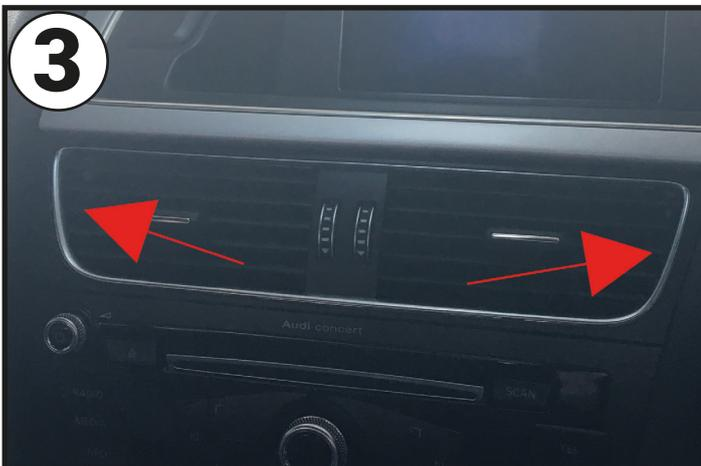
Using a pick tool, insert it in between the fan blades and release the spring clips. Once free, remove and place into storage.
