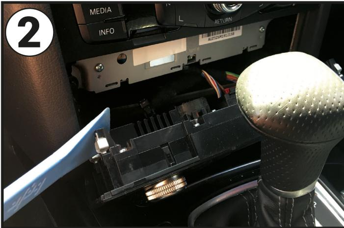
Using the Bojo tool again, pry away and unclip the bottom HVAC panel. Once loose, disconnect the panel connectors and place to one side.
