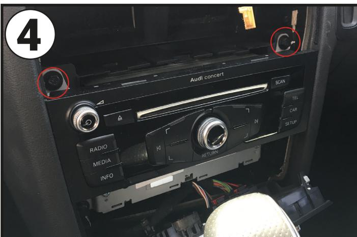
Unscrew the two bolts that hold the head unit into place, when free, remove the head unit and disconnect all the wiring.
