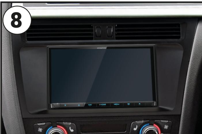
After connecting all the necessary wiring, begin to install the new Double DIN Fascia with the aftermarket head unit into the dashboard. Firmly press down around the edges to ensure it clips into place - this will complete the installation.
