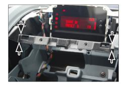
Remove the middle bar (cut at the position marked with arrows)
