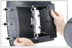
10. Remove clamps from Ford OEM panel. Place clamps on new facia plate
