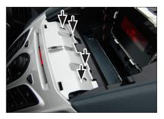
Remove the 4 screws of the OEM head unit
