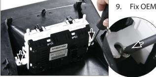
9. Fix OEM display with 2 screws
