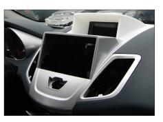
12. Connect all required circuit points of Double-DIN Navigation, mount it to Double DIN facia plate, place it on the dashboard.
