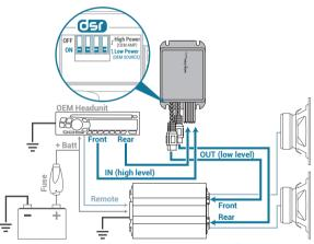
DSR: DOUBLE STEP-DOWN RATIO, allows correct level interfacing with OEM Headunit or OEM Amplifier by switch selection.
