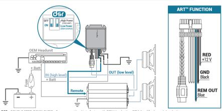
DSR: DOUBLE STEP-DOWN RATIO, allows correct level interfacing with OEM Headunit or OEM Amplifier by switch selection.
