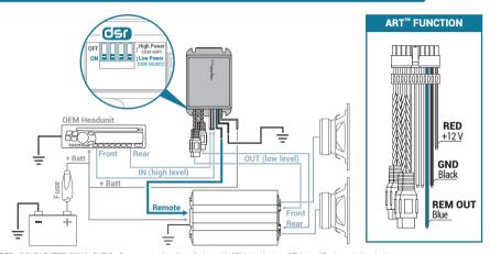
DSR: DOUBLE STEP-DOWN RATIO, allows correct level interfacing with OEM Headunit or OEM Amplifier by switch selection.
