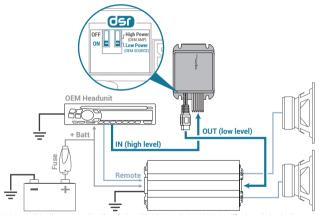
DSR: DOUBLE STEP-DOWN RATIO, allows correct level interfacing with OEM Headunit or OEM Amplifier by switch selection.
