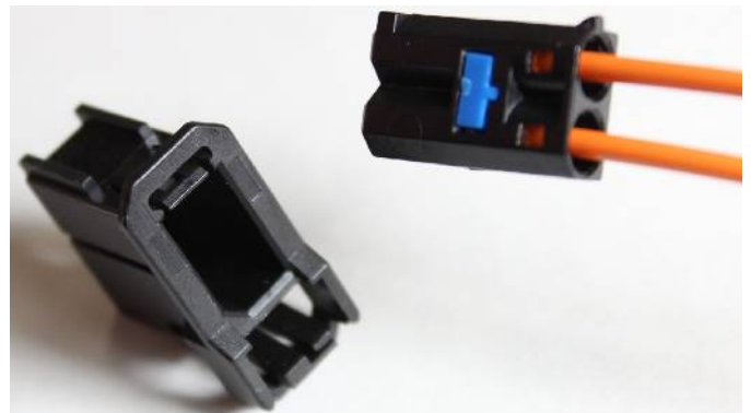
6. Put aside main factory fiber-optic Connector and push sub connector into Supplied GROM connector
